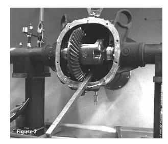
10. Remove differential case. It may be necessary to use a pry bar as shown in Figure 2. Exercise caution when prying on the carrier so that the gasket sealing surface is not damaged. Place shims/adjuster nuts and bearing cups with their respective bearing cap.
