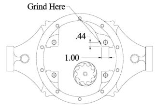
Chrysler 8-1/4 applications require modification to the axle housing as shown to provide clearance for the differential case. Clean housing after grinding.
