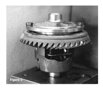
26. Using new ring gear bolts, alternately tighten each ring gear bolt to the proper torque:
