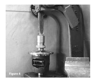
19. Install the differential bearing cones onto the bearing hubs of the differential case using the proper installation tool. See Figure 4.
