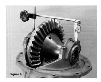
42. Install indicator as shown in Figure 6. Tighten RH adjuster nut until a case spread of .008 - .012 is measured. Rotate drive pinion several times in each direction to seat the bearings and to be sure that binding does not occur. It may be necessary to readjust the case spread by tightening the RH adjuster nut.
